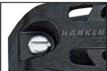
Using block as template, mark holes using a centerpunch. Remove block and drill holes using a 1<sup>3</sup>/<sub>64</sub>" (5.2 mm) drill. Bevel top of deck holes using a small knife to allow sealant to mass. Through-bolt block using recommended stainless steel fasteners, washers and locknuts.
